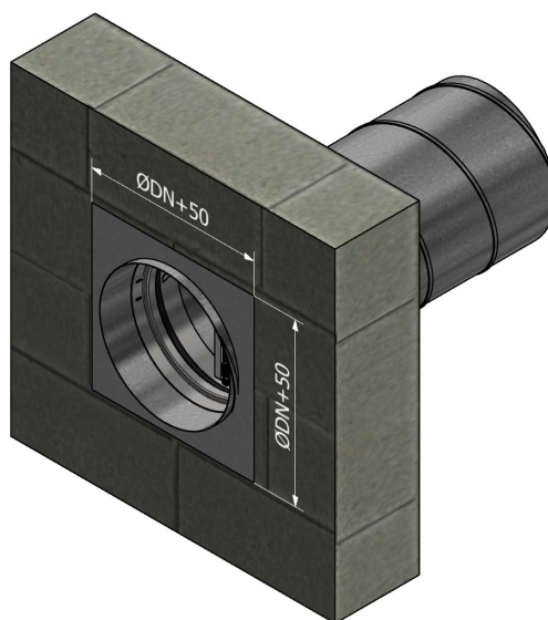
Fig. 15. FDA-BU-KW / FDA-BU-KN, fire damper - dimensions of the sealing of the duct-partition system.
