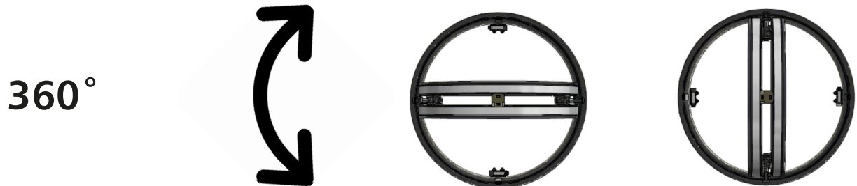
Fig. 6. FDA-BU, fire damper. - blade positions allowed.
