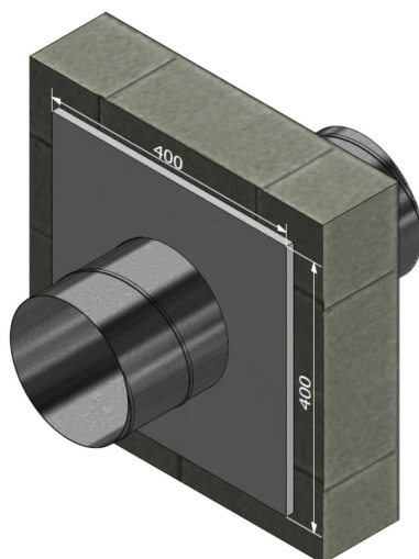
Fig. 12 FDA-BU / FDA-BU-E, fire damper. - dimensions of plasterboard 12.5 mm.
